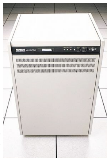
VAX-11/750 introduced in 1980 - the industry's first Large Scale Integration (LSI) 32-bit minicomputer. (Digital Computing Timeline)
