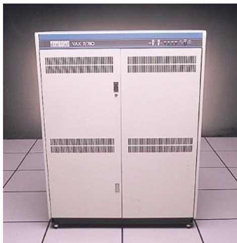
VAX-11/750 introduced in 1980 - the industry's first Large Scale Integration (LSI) 32-bit minicomputer. (Digital Computing Timeline)
