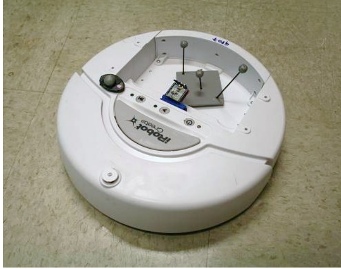
Figure 4-11: iRobot Create with xBee-PRO wireless serial module connected
