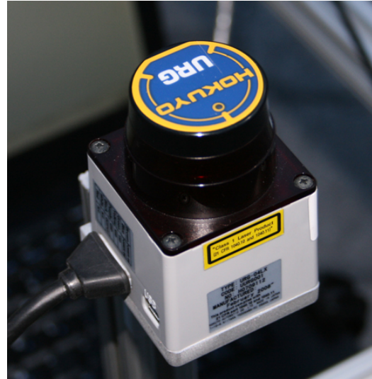
(e) URG-04LX — 4m range, 240^\circ FOV, 0.36^\circ angular resolution, 10Hz update rate
