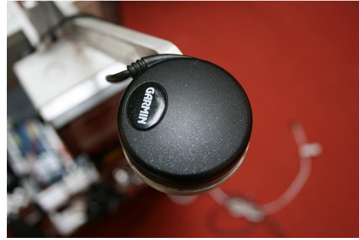
(c) Garmin 18X-5Hz GPS Receiver — 15m resolution, 5Hz update rate
