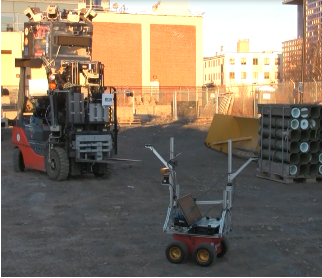
Figure 5-1: Agile Robotics forklift and rover
