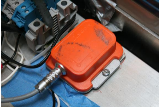
(b) Xsens MTi IMU — 0.05^\circ angular resolution
