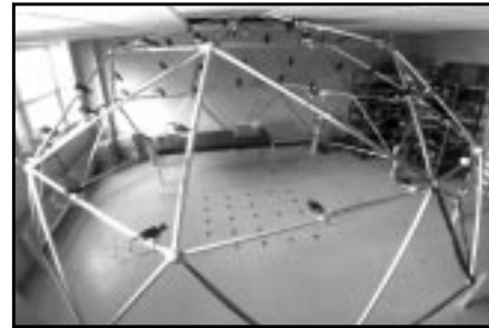
Figure 1: Virtualized Reality 3D Dome camera configuration: 51 cameras are distributed on a hemispherical structure, 5 meters in diameter
