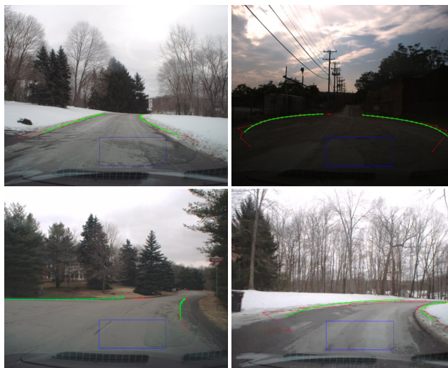
Fig. 1: Sample images of road without road-markings and the outputs of the proposed algorithm. A self-driving car should be capable of driving on roads like the ones appearing on these images. To do so, it is necessary to identify the boundaries of drivable regions. Red lines represent the outputs of our boundary detection algorithm and green lines depict the outputs of our boundary tracking algorithm.
