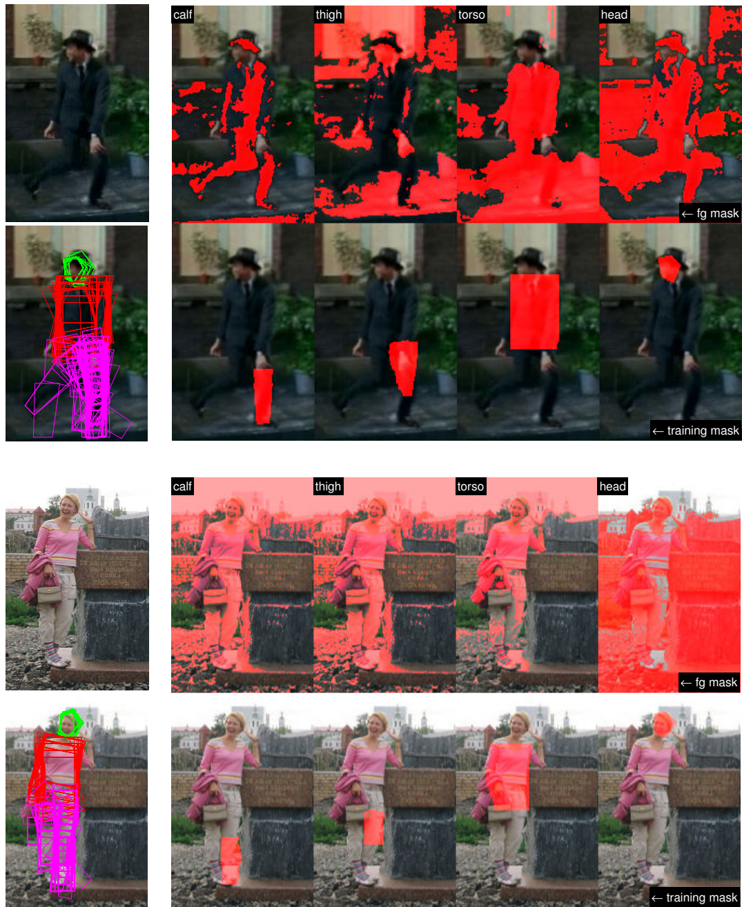
Figure 5.6: Example foreground classification based on DP outputs. First, a number of shape samples are computed by backward sampling (left, bottom). Then, weighting masks are constructed for four parts {calf, thigh, torso, head} respectively (right, bottom). Finally, four discriminative classifiers are learned using weighted training pixels, and applied to the original image to obtain binary foreground masks (right, top). Both weighting and foreground masks are modulated onto the red channel of the original image.
