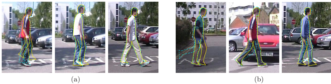
Figure 3.13: Some cases where discrepancies exist between the mean (solid yellow) and the maximum (dotted cyan) a posteriori of the SMC output. (a) Maximum (mode) is significantly better. (b) Mean is significantly better.
