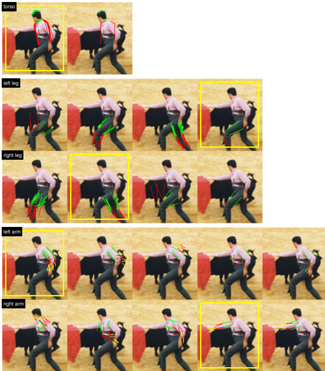
Figure 5.11: Complete candidate sets on 20 example images. Candidates are clustered into \{2, 4, 4, 5, 5\} hyper-modes for \{\text{torso, left leg, right leg, left arm, right arm}\} respectively. These hyper-modes are sorted based on a combination of likelihood and blob/ridge scores. “Preferred” hyper-modes are marked by yellow frames. The ideal automated scoring function would have the top-ranked hyper-mode (leftmost in each candidate set) coinciding with the preferred hyper-mode.
