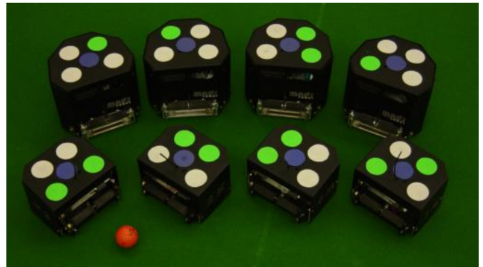
Fig. 1. The CMDragons'02 Robots. Note the tracking and identification pattern on the top of each of the robots.
