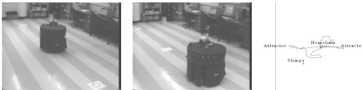
Fig. 11. A Denning robot, Ren, demonstrates the Forage task (left). Ren tags an attractor (center). Telemetry from the Single-Agent Forage demonstration is shown at right. Home base is in the center. Two attractors are located on the left and right. The inactive robot Stimpy is in the lower left.
