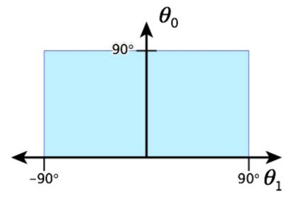
Configuration Space: robot's internal state space (e.g. joint angles)
