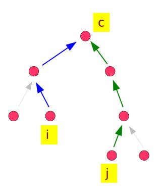
Search upward from i to common frame c, forming  $T_{ic}$ .
