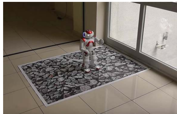
Figure 1: An example target used frequently in AR applications (target is provided as part of Vuforia SDK)
