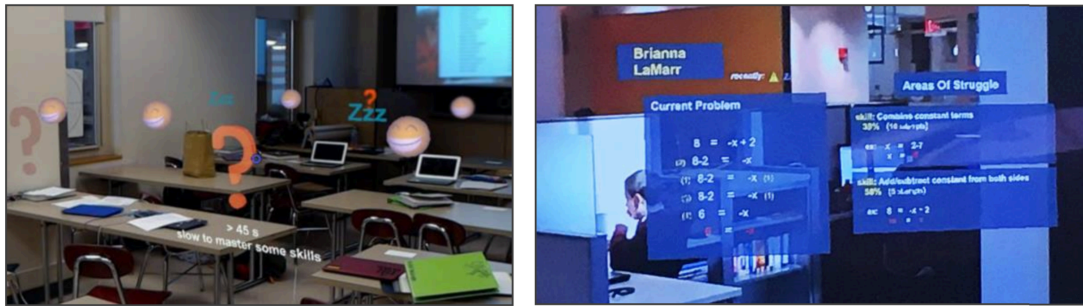
Figure 7. Point-of-view screenshots from teachers using Lumilo (from Holstein, Hong, et al., 2018). Left: A teacher’s view of student indicators, immediately following a pilot study in a live classroom. Right: A teacher’s view of a classroom while wearing Lumilo (with no students present in the room).
