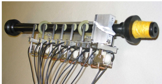
Figure 2.4. Chanter is mounted on aluminum block along with electromagnetic coils that open and close sound holes using rubber pads at the end of lightweight plastic tubes.
