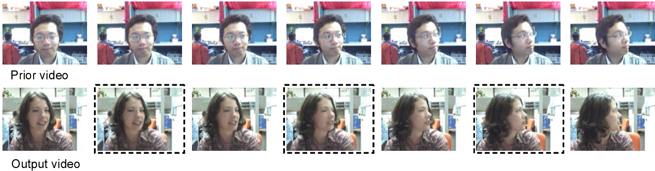
Figure 10. Result of frame rate recovery using the motion field prior. By transferring the motion field from the prior video, intermediate frames (within dashed boxes) that appear seamless can be synthesized. Note that here we are doubling the frame rate.
