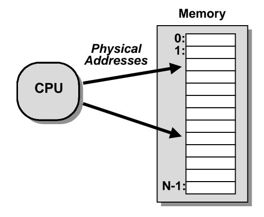
Addresses generated by the CPU point directly to bytes in physical memory
