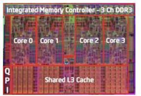
Multiple processors operating with coherent view of memory
