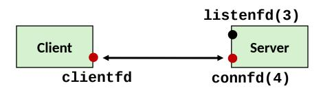
3. Server returns connfd from accept. Client returns from connect. Connection is now established between clientfd and connfd
