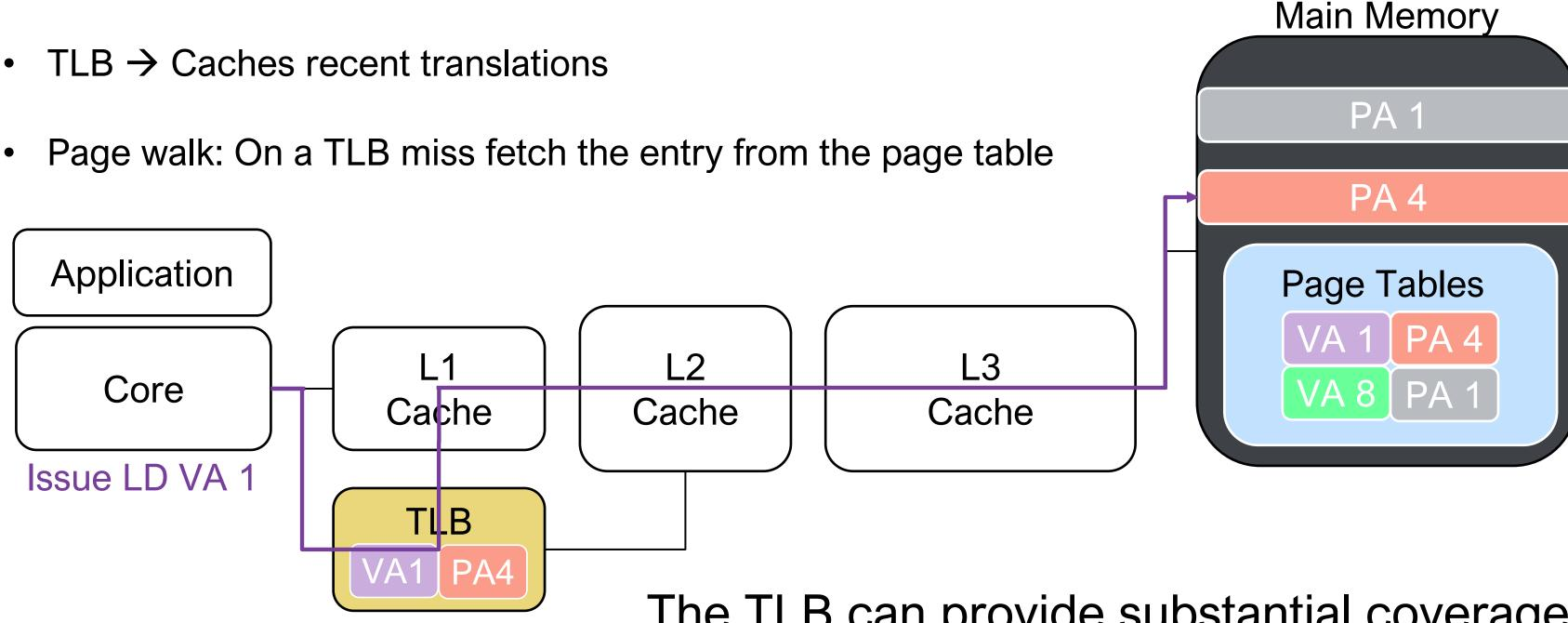
The TLB can provide substantial coverage!
