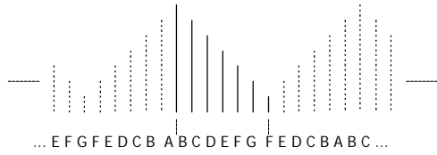
Figure 3. Periodic symmetric extension of the signal ABCDEFG. (It has been assumed that A > B > \dots > G for illustration purposes).
