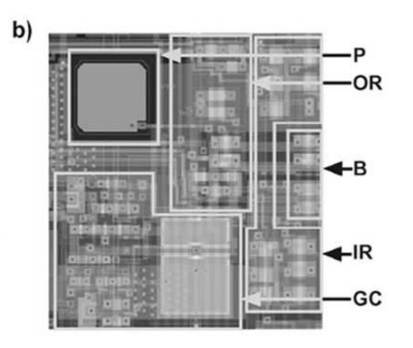
P: photoreceptorOR: outer retina circuitryB: bipolar cellsIR: inner retina circuitryGC: ganglion cells
