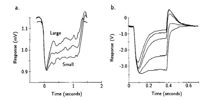
Left: bipolar cell responses in the salamander. Right: output of a pixel in the silicon retina.
