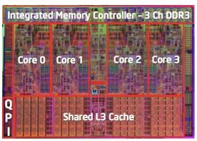
Multiple processors operating with coherent view of memory
