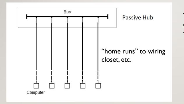
The bus remains an equivalent collision/contention domain, but the wiring gets easier, physically.
