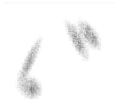
Figure 2: A plot of the estimated density based on a kd -tree; the thin white lines correspond to gaps between leaf nodes of the kd -tree, i.e. regions between neighboring bounding boxes.
