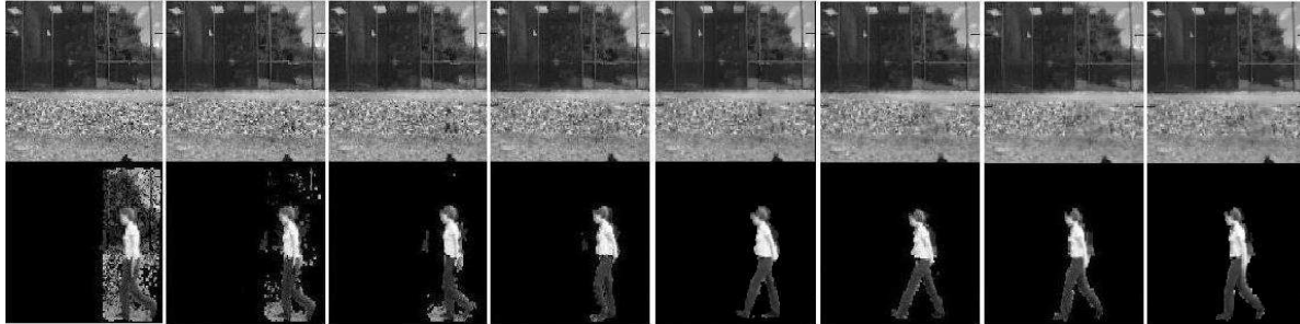
Optimized appearance models for background (top row) and foreground (bottom row). Note that the excessive regions of the crude initial foreground appearance get washed away very quickly.
