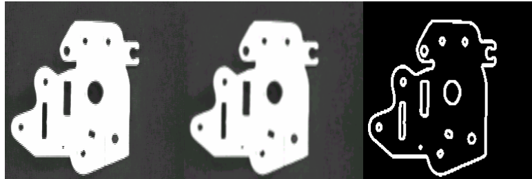
Figure 5: (Left) An industrial object - door part manufactured for automobile industry; (Center) Image after low-pass filtering; (Right) Image after edge extraction.
