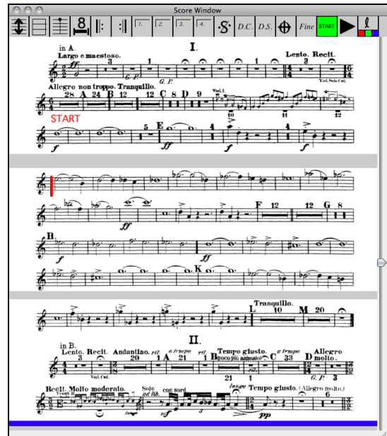
Figure 4. Audio database is accessed through a common music notation interface. The user has selected the beginning of system 3 as a starting point for audio playback, and the current audio playback location is shown by the thick vertical bar at the beginning of system 4.
