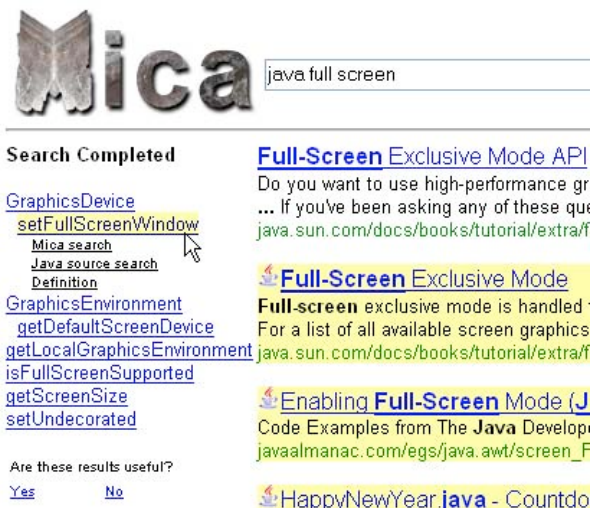
Figure 1. The Mica web application. Mica includes a keyword sidebar on the left, which is generated from web search results shown on the right. Search result pages are categorized by their content; the Java icon indicates that those results contain code.
