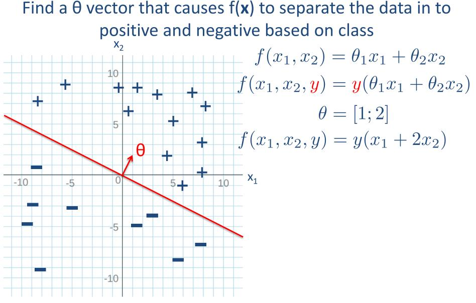
Note: We added y = ±1 to the function to make any correct classification have an f(x, y) > 0
