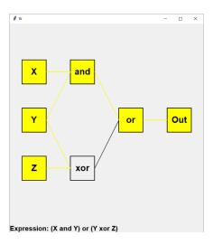
In this project, you will build a simple circuit simulator that can take a boolean expression in text format, generate an interactive circuit for the expression using simulation, and create a truth table for the expression automatically. This will allow you to explore what different boolean expressions output. Note that this project uses **recursion** and **trees** - you should be comfortable with those topics before attempting it!
