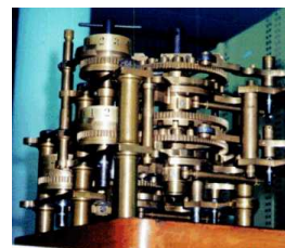
fragment made by H.P. Babbage from parts of Difference Engine No. 1
