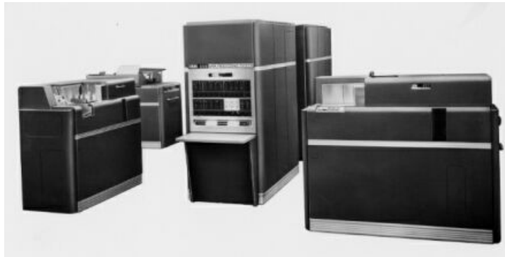
This "white room" view of a 650 installation shows an IBM 533 Card Read Punch in the foreground at left; the 650 Console Unit at center, with an IBM 655 Power Unit behind it; and an IBM 537 Card Read Punch at right. (IBM Archives)
