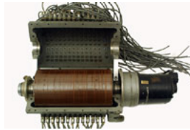
ERA Magnetic Drum (left), English Electric Magnetic Drum (right)
