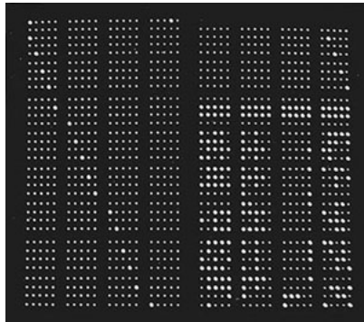
display from a Display Cathode Ray Tube for a Williams-Kilburn CRT Store from a Ferranti Mark 1 (University of Manchester)
