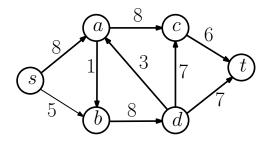
Run Ford-Fulkerson, drawing the **residual network** at every step, and show the final residual network. What is the maximum flow? What is the capacity of the minimum cut? Partition the vertices into two sets (S, T) such that  $s \in S$ ,  $t \in T$ , and (S, T) is a minimum cut.
