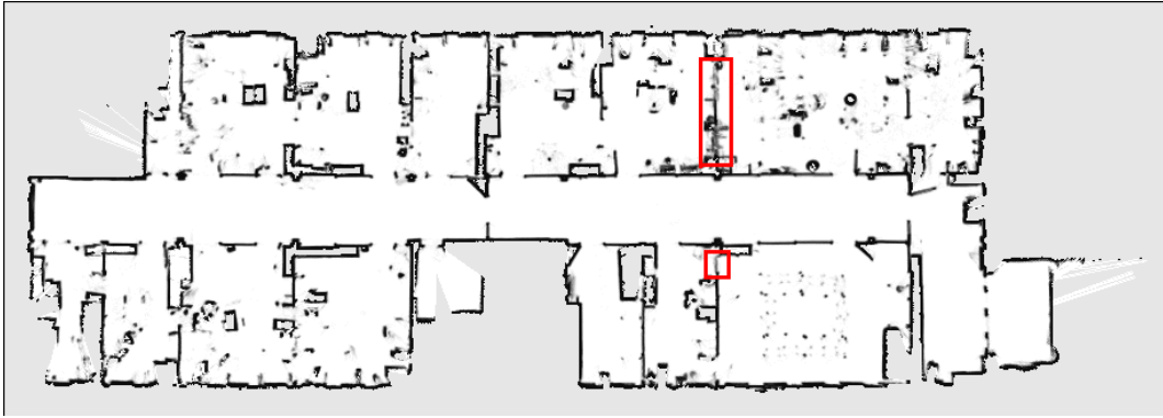
Figure 4: A map produced using a density mapping technique. Regions in red indicate glass walls which are indicated as having partial returns.
