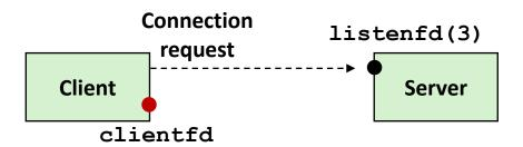
2. Client makes connection request by calling connect
