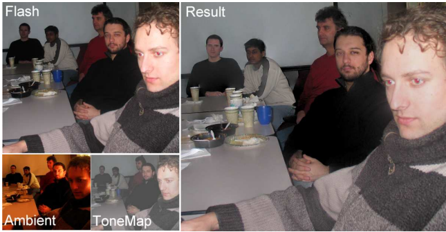
Figure 7: Dinner Table. Non-uniform illumination in a scene with large depth variation. Our method selectively scales the flash image gradients such that the brightness falloff with the distance from the camera is minimized. A direct tone-mapping procedure leads to loss in contrast.
