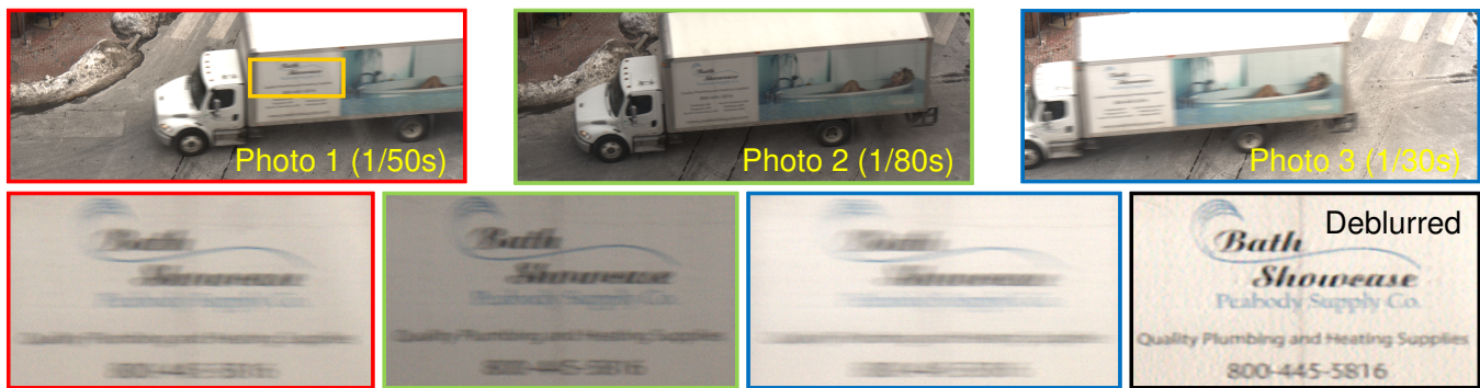
Figure 2: One can use widely available auto exposure bracketing (AEB) mode on consumer grade digital SLR cameras to achieve PSF null-filling. Top row shows three photos of a moving truck captured using Canon Digital Rebel XT with AEB mode (exposures: 1/50, 1/80, and 1/30 sec). Bottom row shows the manually rectified blurred regions and the deblurred output. Notice that sharp features such as text are recovered in the deblurred image.
