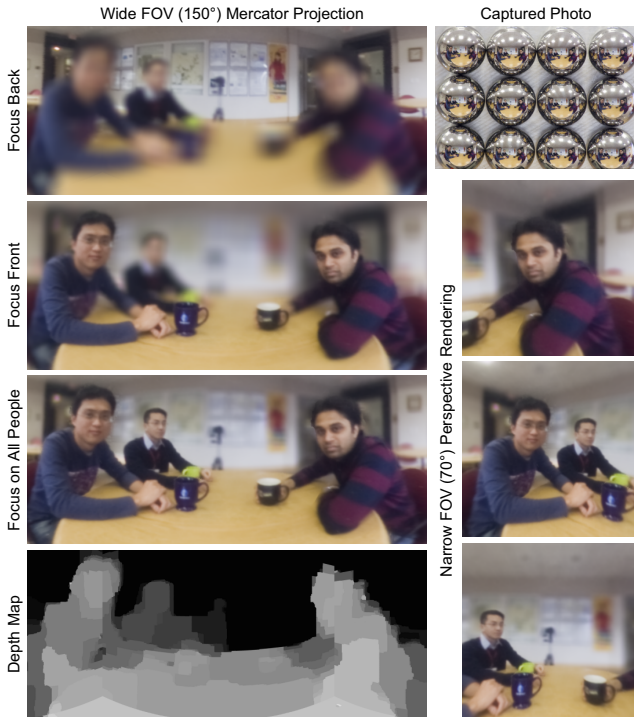
Figure 9: (Left) Depth map estimated from light field can be used to bring all foreground objects (at different depths) in focus. (Right) Captured photo and narrow FOV refocusing results.
