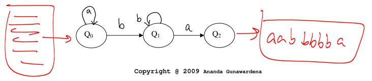
Finite automata (FA) can be built to recognize valid strings defined by a formal language. For example, we can use a machine as defined above to find all substrings that begins with zero or more a's immediately followed by one or more b's and then ending with an 'a'.
