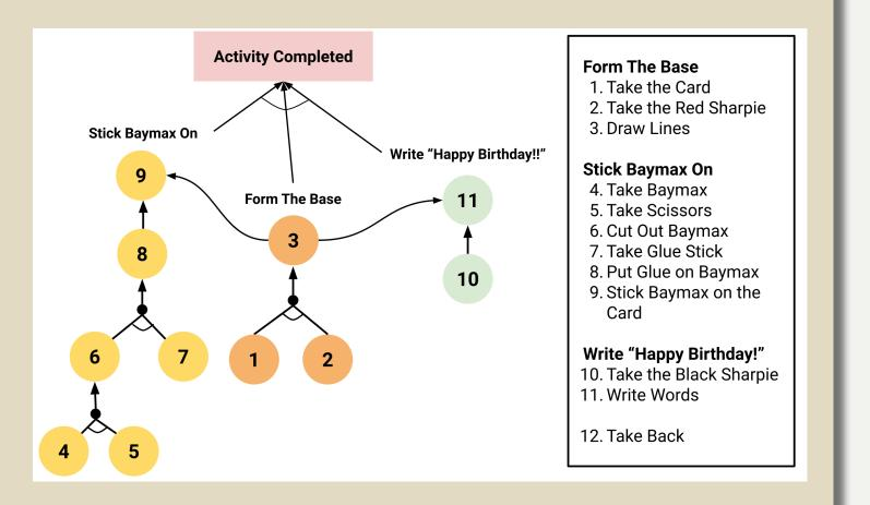
**Fig 2.** The and-or graph representation of our task. Each arrow pointing from node A to B indicates that A must occur before B.
