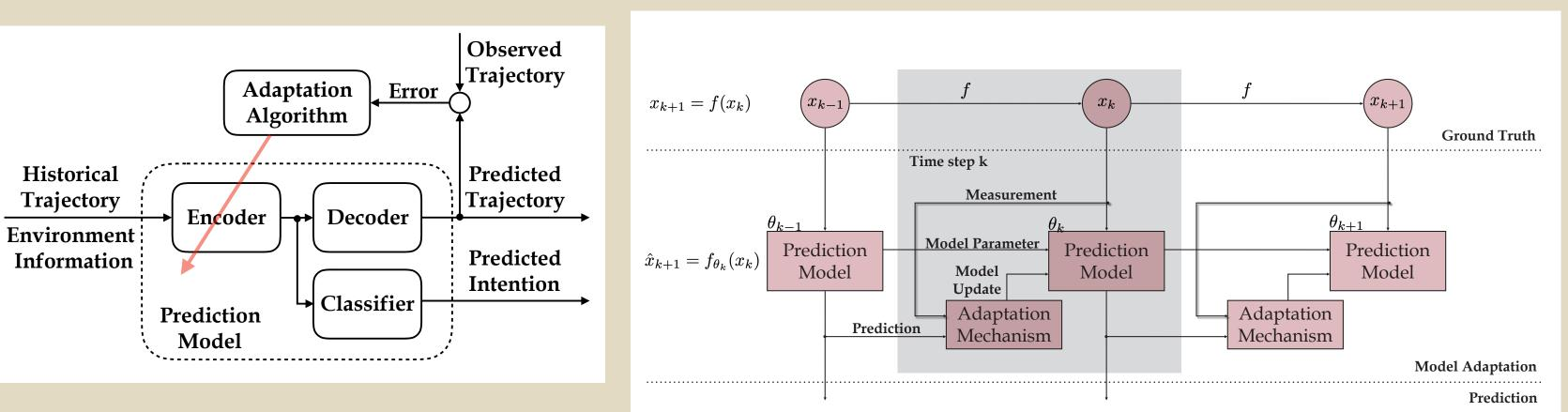
Fig 6. The general framework of the online adaptation system. At every time step, the ground truth is received and the error calculated. The encoder is then updated using the error.
