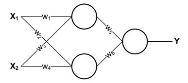
2. (4 pts) Assign proper activation functions (**S** or **L**) for each unit in the following graph so this neural network simulates a binary logistic regression classifier:  $Y = \arg\max_y P(Y = y|X)$ , where  $P(Y = 1|X) = \frac{\exp(\beta_1 X_1 + \beta_2 X_2)}{1 + \exp(\beta_1 X_1 + \beta_2 X_2)}$ ,  $P(Y = -1|X) = \frac{1}{1 + \exp(\beta_1 X_1 + \beta_2 X_2)}$ .
