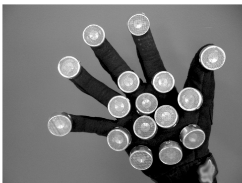
Figure 3. Sound Glove: transducers can work all together as a group creating a larger parametric array or can be split into a sender/receiver configuration.
