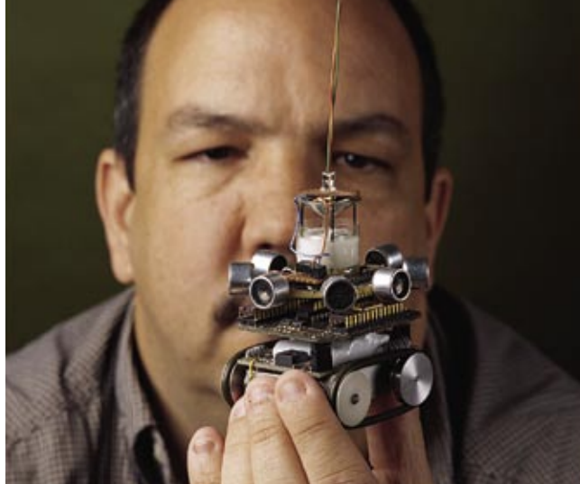
HE'S GOT THE WHOLE ROBOT in his hands: One of the authors (Grabowski) holds a millibot. This particular design is about as small as designers could make it from off-the-shelf components.
