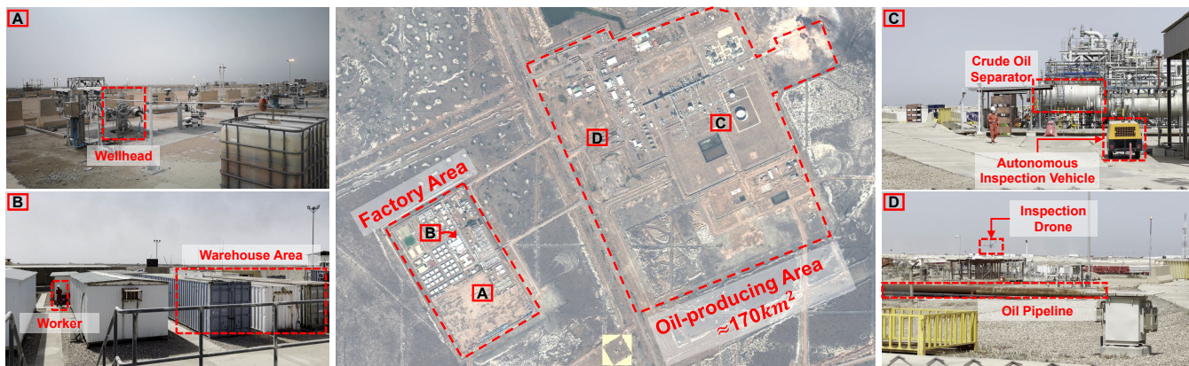
Figure 1: Industrial inspection is carried out by 10 drones and 2 autonomous vehicles in one of the world’s largest oil-field ( >170\text{km}^2 ) in the Middle East. These agents are coordinated by SwarmMap that runs on an Nvidia AGX Xavier edge server.
