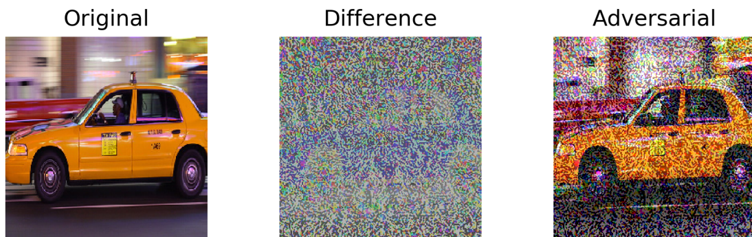
Figure 1.1: Adversarial example of a yellow cab generated using FGSM [Goodfellow et al., 2015]. The original image is correctly classified as a cab with the confidence of 0.999, whilst the adversarial example is incorrectly classified as a jigsaw puzzle with the confidence of 0.629. The adversarial perturbation in this example is discernible, but [Szegedy et al., 2013; Kurakin et al., 2017] contain examples of adversarial perturbations that are hardly recognizable by the human eye. The original image of the yellow cab comes from the ImageNet dataset [Deng et al., 2009], which is publicly available at http://www.image-net.org/ .
