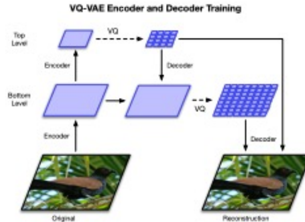
(a) Overview of the architecture of our hierarchical VQ-VAE. The encoders and decoders consist of deep neural networks. The input to the model is a 256 \times 256 image that is compressed to quantized latent maps of size 64 \times 64 and 32 \times 32 for the bottom and top levels, respectively. The decoder reconstructs the image from the two latent maps.
