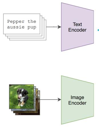
The text encoder (e.g., an encoder-only transformer) and the image encoder (e.g., a ResNet-like CNN or ViT) are both linearly projected into samedimensional vectors i.e., the multi-modal embedding space
