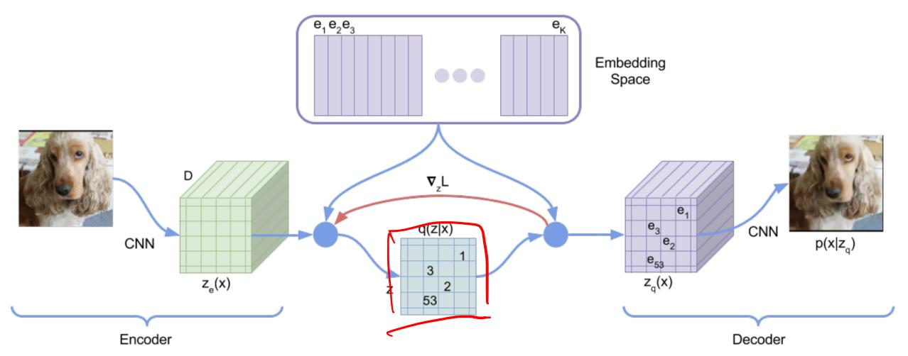
• Treat the gradient w.r.t.  $z_q(x)$  as an estimate of the gradient w.r.t.  $z_e(x)$
