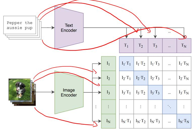
• Given a mini-batch of *N* (image, caption) pairs, both encoders are simultaneously pre-trained to maximize the cosine similarity of corresponding image-caption embedding vectors and minimize all other pairwise cosine similarities
