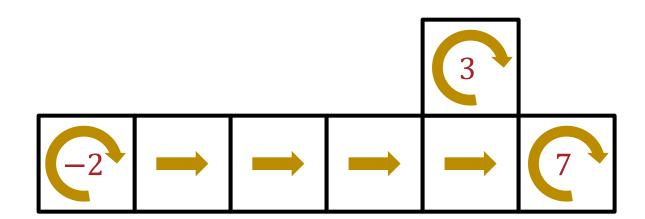
$R(s,a) = \begin{cases} -2 \text{ if entering state 0 (safety)} \\ 3 \text{ if entering state 5 (field goal)} \\ 7 \text{ if entering state 6 (touch down)} \\ 0 \text{ otherwise} \\ \gamma = 0.9 \\ \hline 0 \\ 5.103 \\ 5.67 \\ 6.3 \\ 7 \\ 0 \\ \hline \end{cases}$
