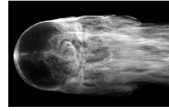
Figure 6: Impulsively started flow past a sphere at Re=15000 simulated using our solver
