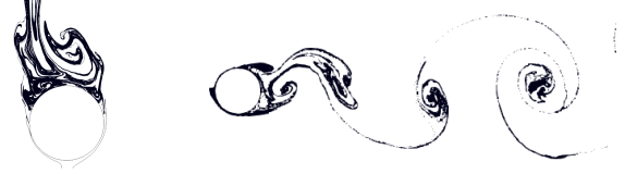
Figure 3: Our method captures the velocity field near the boundary efficiently and with high apparent fidelity. Left: zoom-in near the boundary flow. Right: the entire simulation, Re=15000 .
