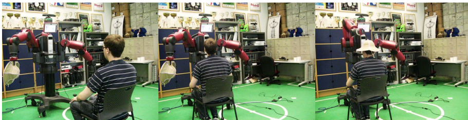
(a) User is initially at an unreachable pose. (b) Robot requests the user to move forward. (c) Manipulator successfully puts hat on the user.
