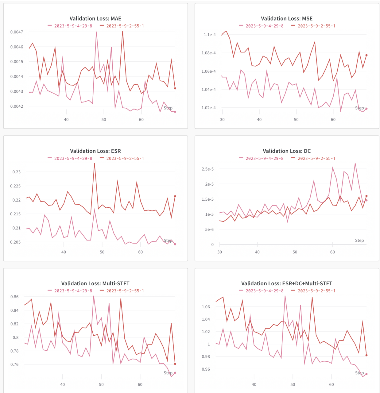
Figure 4.5: Validation loss curves among different models with the same IIR filter order using different audio channels. 2023-5-9-2-55-1's model has 16 audio channels and an order of 4 in the S4 IIR filter. 2023-5-9-4-29-8's model has 32 audio channels and an order of 4 in the S4 IIR filter.
