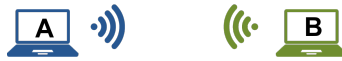
Figure 3: Overview Diagram of Experiment Setup: Device A is running Wireshark, Device B can be any device communicating with Device A.
